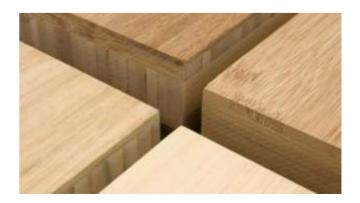
is surprisingly strong, with up to three times the structural capacity as normal timber. Despite this, there remain some concerns about the bamboo's resilience, as it decays more quickly than wood if not treated with the right preservatives.
