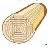
The resulting pattern on the board's surface is called cathedral or crown grain, having pronounced figure as shown in the photos to the left.
