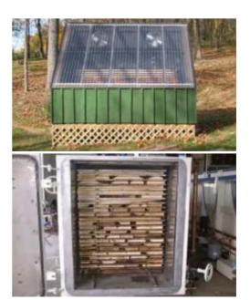
temperature and humidity inside the kiln can be controlled. Proper kiln drying schedules available needs to be followed; care should be given to ensure following the Indian Standards for seasoning (drying) timber (BIS 1993).
