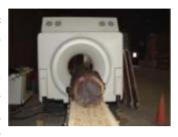
proportion of high-quality lumber that will be produced from that log, and to help buyers and sellers to settle on a fair price. Sophisticated modern mills make use of ultrasound, X-rays etc. capable of detecting internal defects in the logs for grading them.
