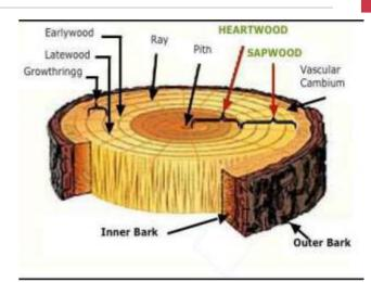
properties of timber used in construction is their strength, specific gravity/wood basic density, moisture content, shrinkage and swelling, colour, grain and odour. Wood was the traditional choice of building material for manufacturing structural beams, doors, windows, wall panelling, flooring and many other applications because of the availability, practicality and appearance.
