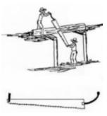
conversion or 'breaking down' of the logged timber, which means rough sawing. Sawmill essentially comprises the facility where logs are cut into lumber. Modern sawmills uses power operated motorized saws to cut logs lengthwise to make long pieces, and
