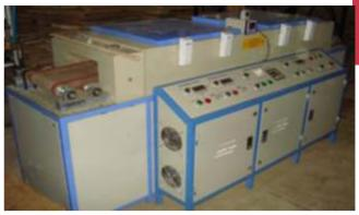
for precise vapour pressure control. Process leaves the wood incredibly stress free with no need for conditioning.
