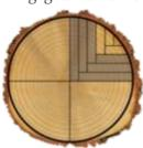
boards successively along the axis. Quarter Sawing involves sawing in a plane which is to be more or less perpendicular to ray and perpendicular to the growth ring of the tree; used for decoration piles and for surface cracked wood. This method produces the most stable and desirable grain patterns.
